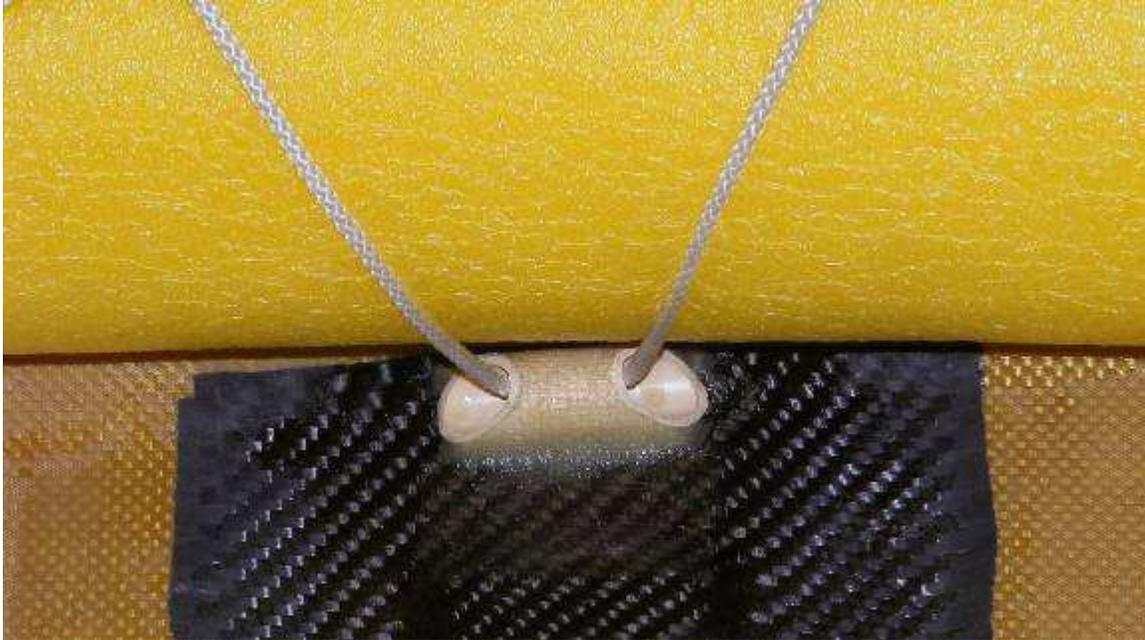
Photo: A pipe tie-in fixture is bonded with fiberglass to the carbon rib of a Kevlar hull. Fiberglass has been trimmed from pipe holes and flotation is lashed in place.
