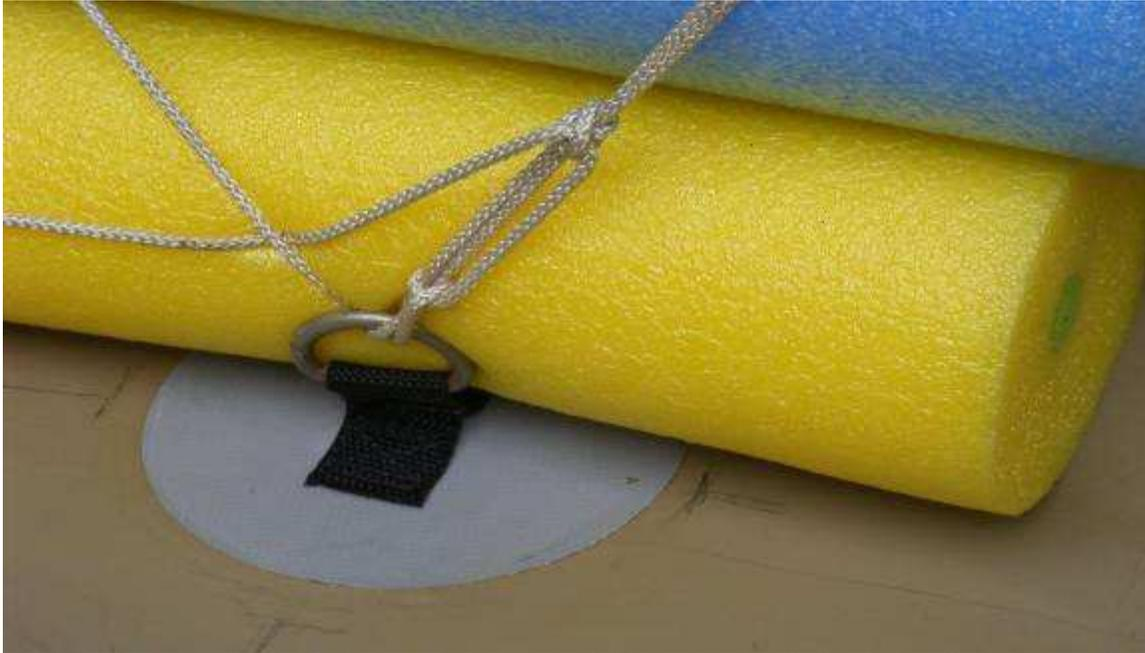
Photo: D-ring patch installed in ABS Royalex hull. Lacing is 1/8" nylon rope.
